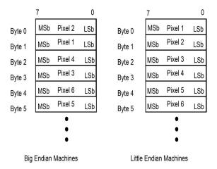
The DICOM standard specifies that the first pixel byte should be set to the *least significant byte* of the OW value. The next pixel byte should be set to the *most significant byte* of the OW value.
