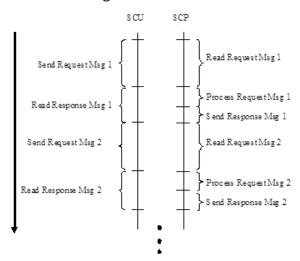
When asynchronous operations are negotiated, the SCU can poll for a response message, but if a message is unavailable, it can start sending the next request message right away (if the max operations will not be exceeded). This allows an SCU to utilize the network bandwidth more fully. There is only a small time when the SCU polls for a response message during which data is not being sent from the SCU to the SCP.
