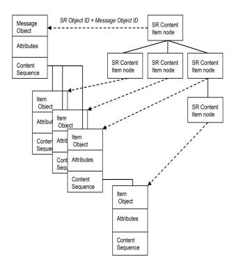
When a message or item object is mapped with the SR object, it is marked with a special flag that prohibits some of the operations that can break the structured report hierarchy. For example, MCattributeSet.duplicate() will not work on the messages mapped with the SR object.
