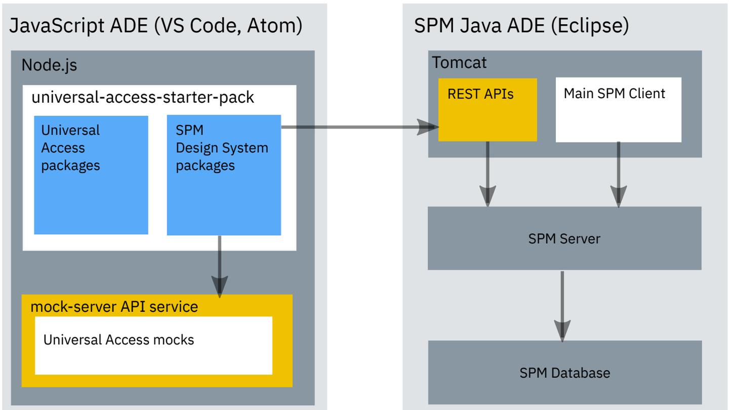
Figure 3. SPM React and Java application development environments
